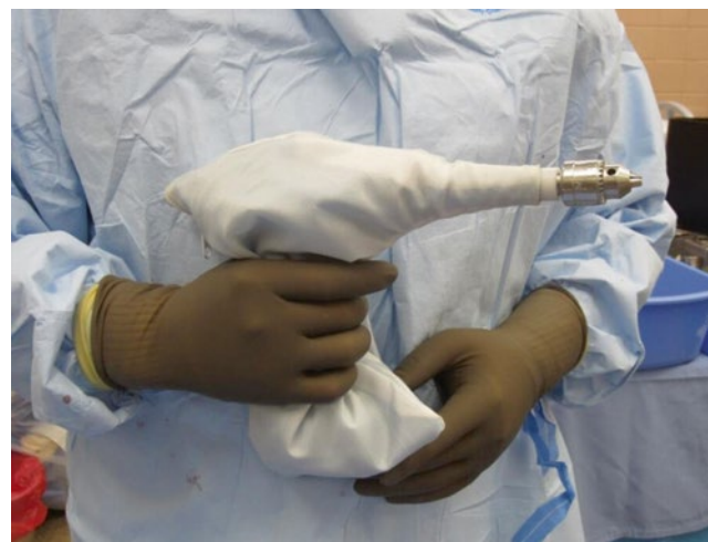
Fig. 14.6 Cordless drill kit shown with sterile cover and surgical chuck
