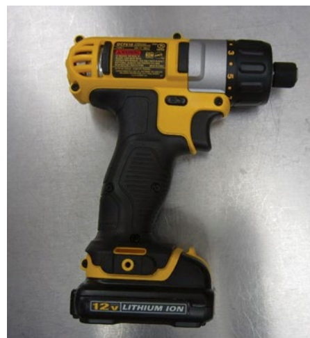
Fig. 14.5 12v cordless variable-speed drill
